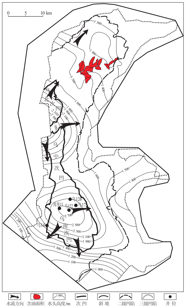
图 1 海拉尔盆地乌尔逊凹陷中部含水岩系沉积水动力场 Fig. 1 Hydrodynamic fields of water-bearing rock series in central Wuerxun Sag, Hailaer Basin
