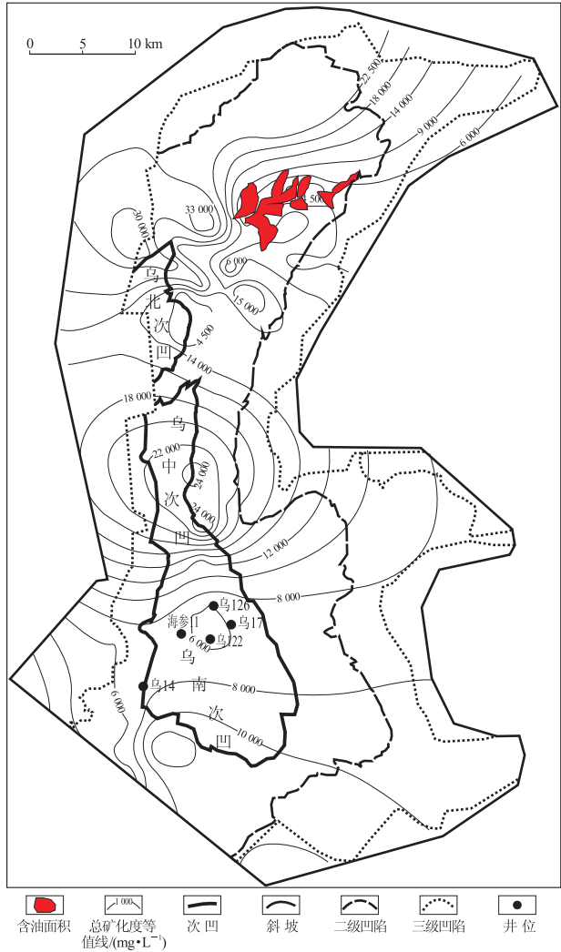
图2 海拉尔盆地乌尔逊凹陷中部含水岩系矿化度等值线 Fig.2 Salinity contour map of water-bearing rock series in central Wuerxun Sag, Hailaer Basin
