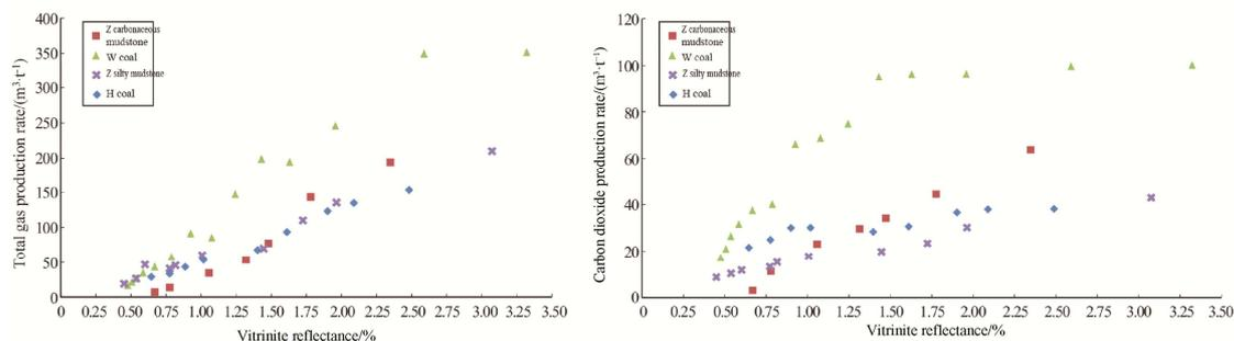
**Fig. 1** Evolution characteristics of total gas and carbon dioxide production rates of source rocks in coal measures
