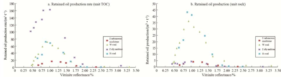
**Fig. 4** Retained oil production rate and production curves of source rocks in coaly formations
