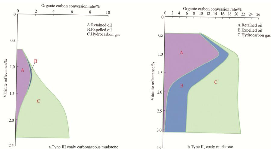
**Fig. 7** Models for hydrocarbon generation, expelling, and retention in coaly mudstones and carbonaceous mudstones
