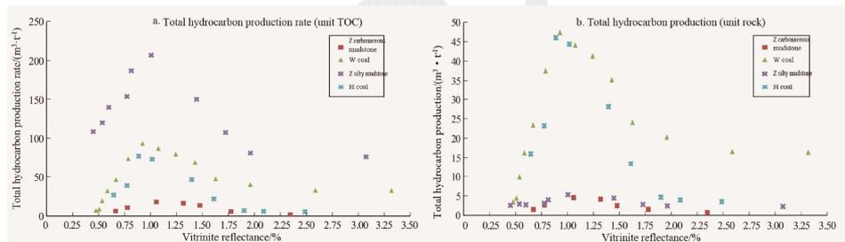
**Fig. 5** Total hydrocarbon production rate and production curves of source rocks in coaly formations
