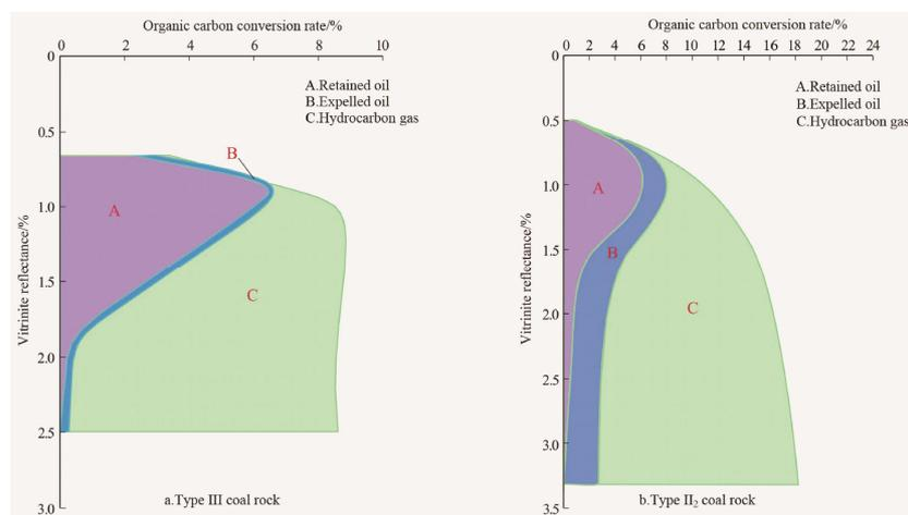
**Fig. 6** Evolution models for hydrocarbon generation, expelling, and retention in coaly source rocks
